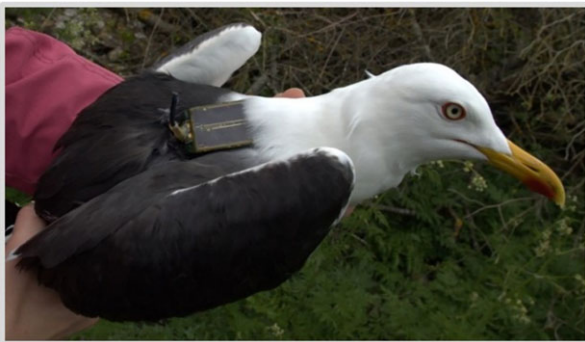
Figure 3. Lesser black-backed gull ( Larus fuscus ) equipped with an 18 g solar-powered UvA-BiTS device (size: 61 \times 25 \times 10 mm). The GPS unit used is the Lea-4S chip from U-blox manufacturer. See [42] for UvA-BiTS detail. Photographic credit: the authors. (Online version in colour.)
