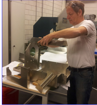
FIGURE 3.4: The “bird cages”. Jan Kalwij from the workshop bending the “bird cages”. The inner and outer boxes used to insulate the oven and the heated Zeeman slower window assemblies.
