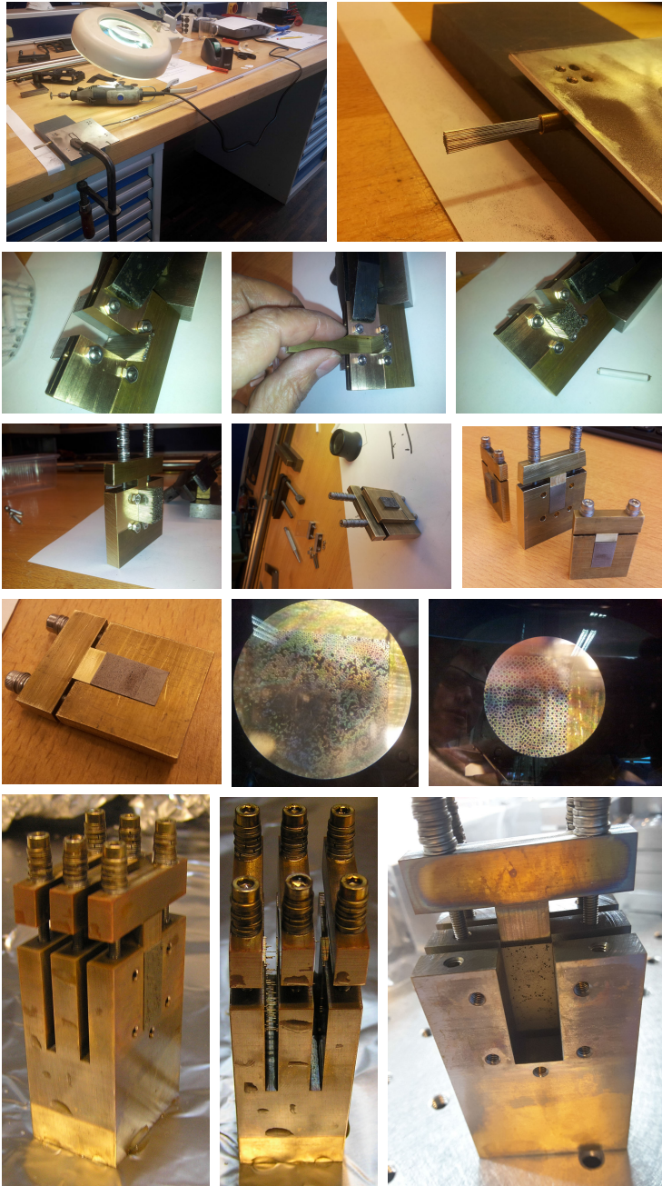
FIGURE 3.9: Strontium Continuous Atom Laser machine. Jig used to hold the microtubes in the wire cutting machine in order to cut the microtubes to length. Approximately 10-20% of the tubes slid out of the holder during the cutting process in the wire cutting machine. This significantly complicated the loading process as the bad tubes needed to be removed from the array by tweezers, a particularly labour intensive process.
