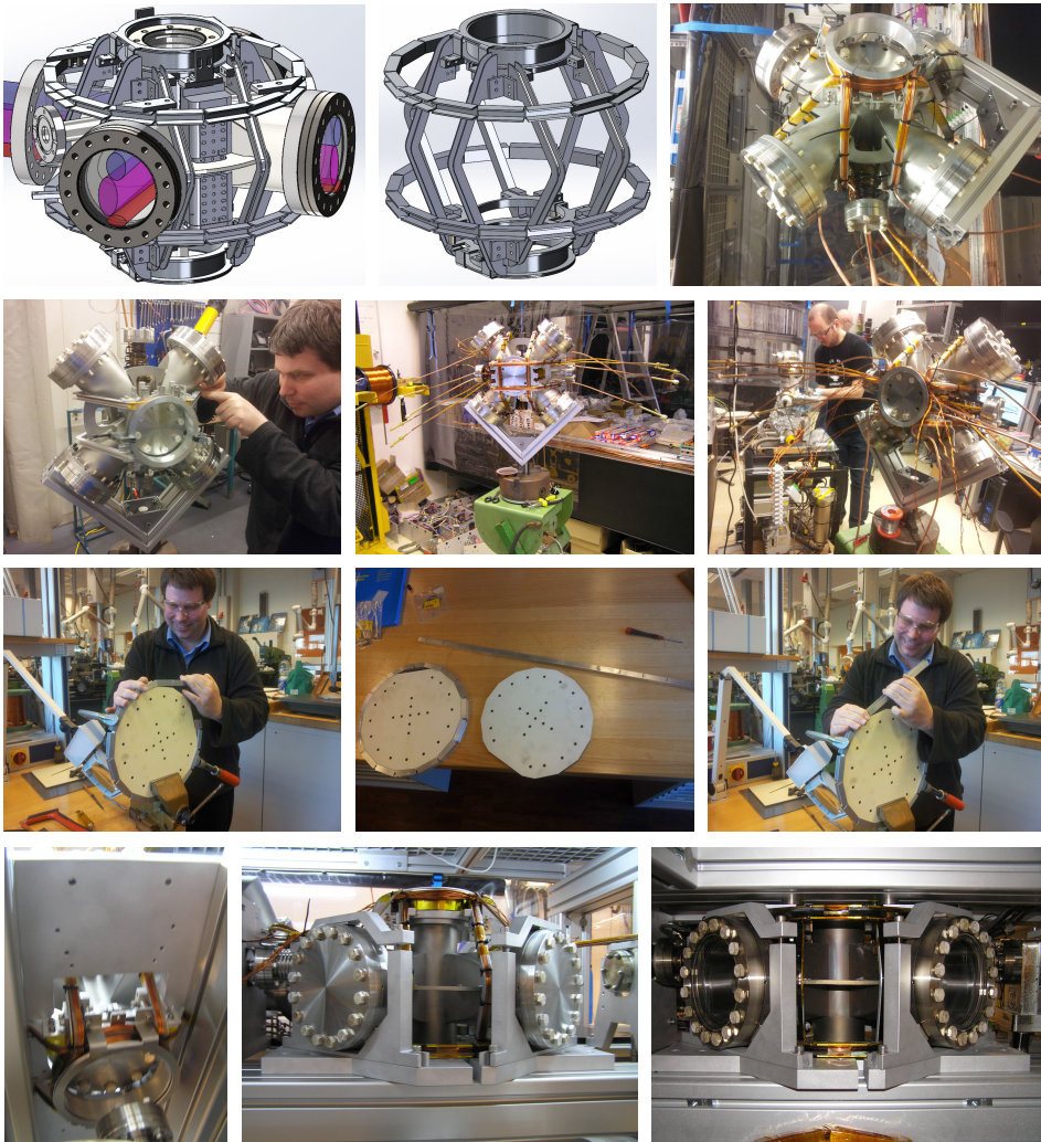
FIGURE 3.37: Design and construction of the bias coils. Here we show the design and construction of the bias coils around the 2D MOT chamber.
