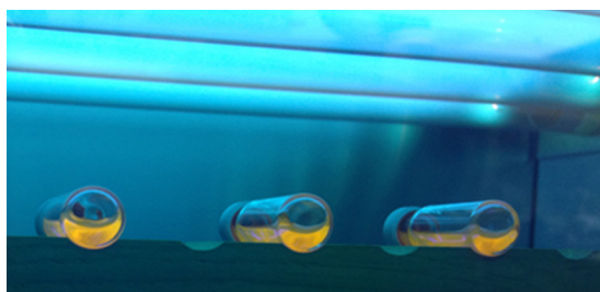
Fig. 1. Photographic image of the setup for exposure of the dye solutions to the UV light.
