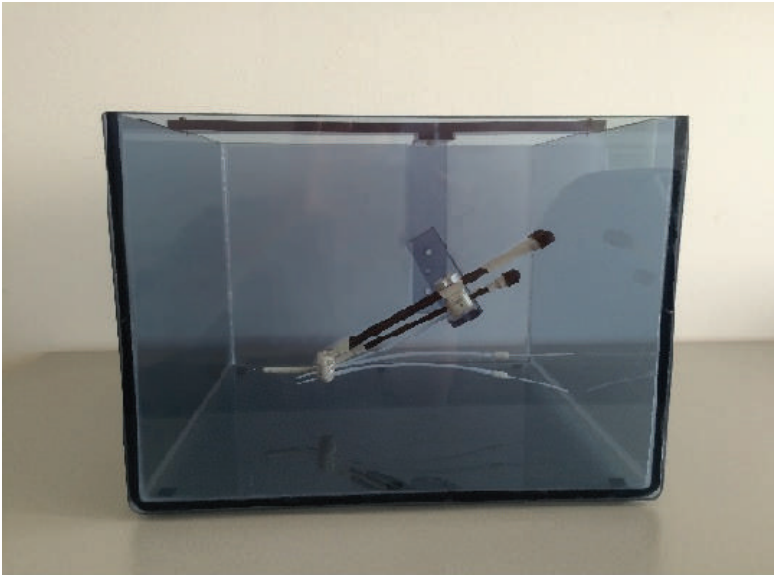
Fig. 1 The MR-compatible phantom in which the Utrecht applicator is suspended.
