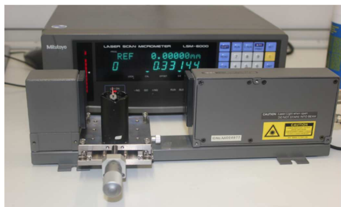
Figure 1. Travel cross roller table connected to a micrometre perpendicular to the scanning laser beam of a laser scan micrometer. D_0 level was established as a first reading achieved by LSM, where the specimens touched the laser beam; consequently, specimens were moved manually using micrometre ruler for further measurements
