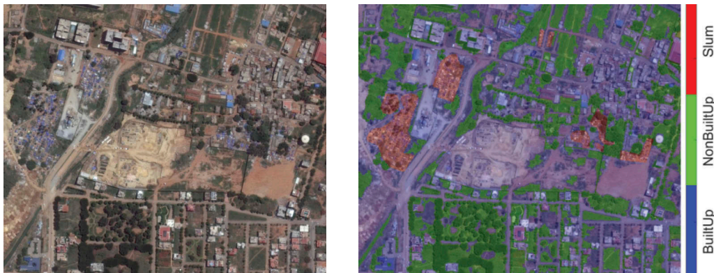
Figure A1. Bangalore ROI 1. Left: original image and Right: overlaid ground truth for slums, non built-up (mostly vegetation) and the remaining areas (built-up).
