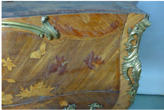
Figure 14 Detail commode, two mounts are removed, which exposes brighter coloured tulipwood and purpleheart.
