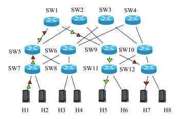
Fig. 5. An example of partial Fat Tree network (Li et al. 2014).
