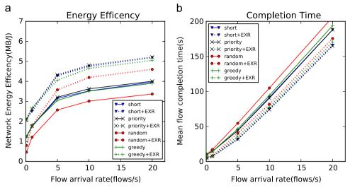
Fig. 8. Network energy efficiency and mean flow completion time against the arrival rate of large flows (5 GB) in the Fat Tree network.
