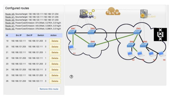
Fig. 3. A screen shot of the topology and the configured routes in the emulated network environment.
