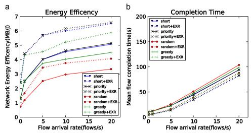
Fig. 6. Network energy efficiency and mean flow completion time against the arrival rate of large flows (5 GB) in the BCube network.
