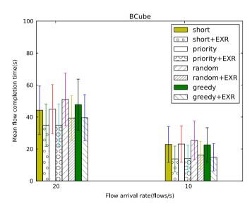
**Fig. 7.** Mean flow completion time with standard error against the arrival rate of large flows (5 GB) in the BCube network.
