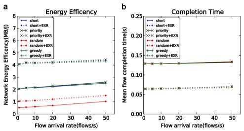
Fig. 9. Network energy efficiency and mean flow completion time against the arrival rate of small flows (64 MB) in the BCube network.
