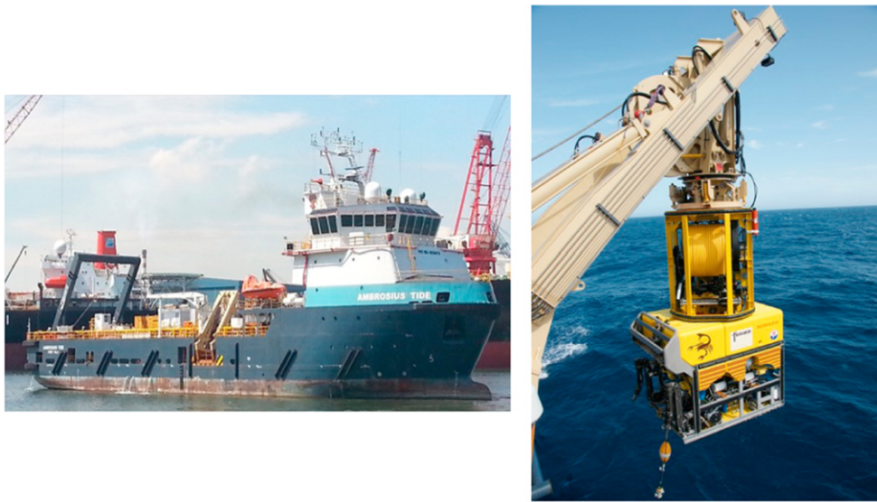
Figure 10. Photograph of the Ambrosius Tide boat, used for the KM3NeT/ARCA string deployment (left). Photograph of the remote operated vehicle, used for the string connection (right).
