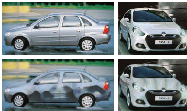
Figure 10. Shape manipulation application. A user has drawn to manipulate the normal map extracted from our indirect approach. The reflectance map and the new normal map can be used to simulate the new shape's appearance.
