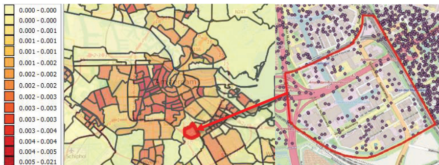
Figure 3. P_{home}(x, y) — personal cars density per ground square meter used to generate agents homes (left) and example of randomly and uniformly populated neighborhood with 165 cars (right).
