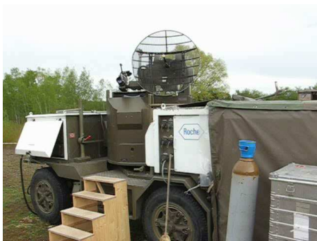
Fig 3: Tracking radar “Superfledermaus” used for validating quantitative measurements by weather radar.
