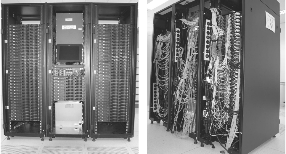
Figure 1.3: The DAS-2 cluster at the Vrije Universiteit Amsterdam, from the front ( left ) and from the back ( right ). Photos courtesy of Kees Verstoep, VU.
