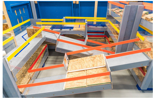
Fig. 3 The smaller scale rapidly manufactured Robot League arena, based on a 30 cm (1 ft) nominal clearance
