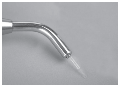
Figure 2. Nd:YAG laser fiber tip emerging out of handpiece tip
