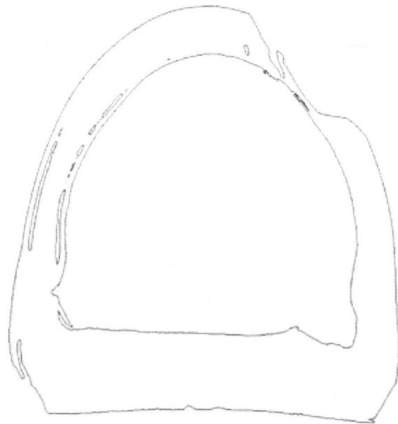
FIG. 10. VOIDS HIGHLIGHTED AFTER EDGE DETECTION IN PARAVIEW.
