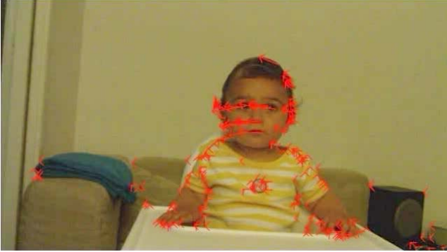
Fig. 11. Example of the optical flow vectors obtained in a frame using the pyramidal implementation of the Lucas and Kanade algorithm [23]. Optical flow vectors are represented as red arrows in the picture.
