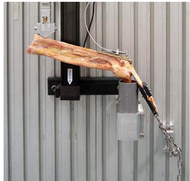
Fig. 4 The custom-made stepper motor actuated testing bench setup. The humerus is potted into a polyvinyl chloride pipe and the triceps tendon is secured with clamp and mounted on the bench. The DVRT is placed across the fracture at the posterior aspect of the olecranon. A bending moment is achieved at the osteotomy site by the actuator at the distal ulna
