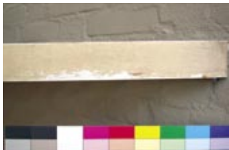
2. Discolouration and abrasion of gelatine layers on the 1976 chromogenic RC-paper with a silkscreen structured surface typical of the 1970's.
