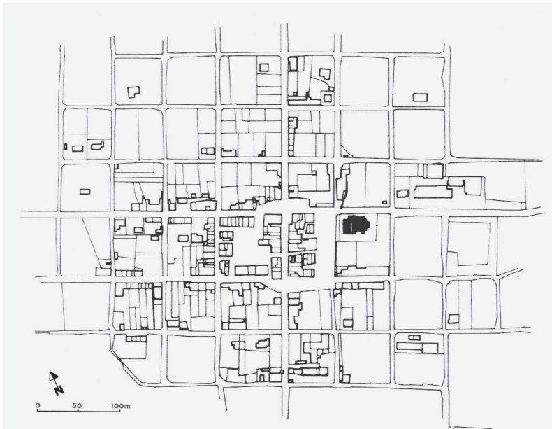
fig. 2.54: Plan of Saint-Denis-de-Saissac. (From: Lauret, Malebranche & Séraphin 1988) The town was founded by the French crown between 1290 and 1293. The orthogonal structure of blocks surrounded by streets is larger than the actual town, extending much further than this plan shows. (see fig. 2.55)
