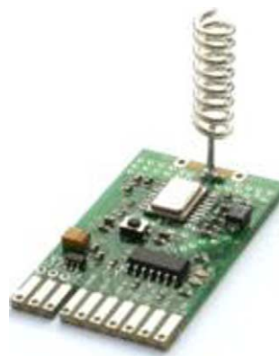
Fig. 6. Wireless network node to which sensors can be attached.
