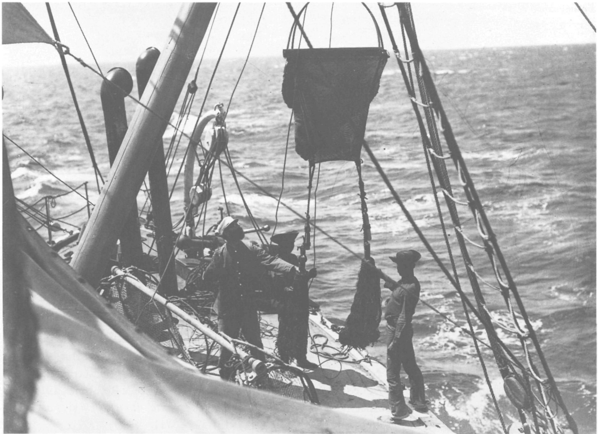
Fig. 14. Lowering the dredge.
