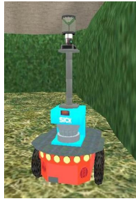
Fig. 7: OmniP2DX, with the omnicam sensor high above the Sick laser range scanner.
