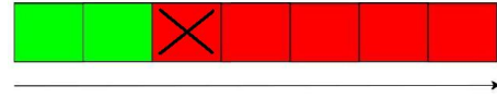
(a) Example where N = 4 : The pixel with an 'X' has been classified as a hit point because N pixels behind it are classified as non-free space pixels.
