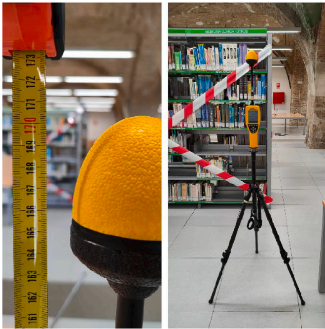
Fig. 3. Used Narda NBM-550 broadband field meter and isotropic Narda EF0691 probe (right) and height of measurements (left).
