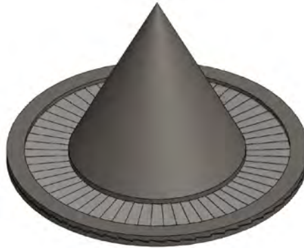
Figure 4-4 Schematic of a single row blade distributor. Source: Figure created by author.
