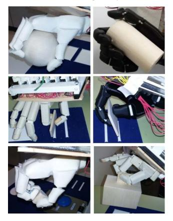
Figure 7. Tested hands performing SHAP's LAO tasks. The six objects of the LAO set are shown.
