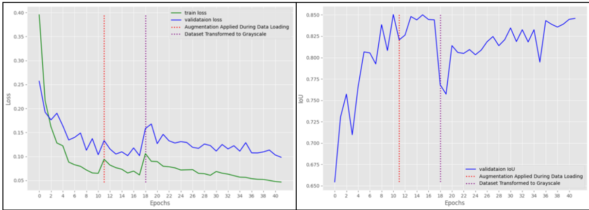
Figure 3.8 – Model-G Convergence and Validation IoU over 42 Epochs
