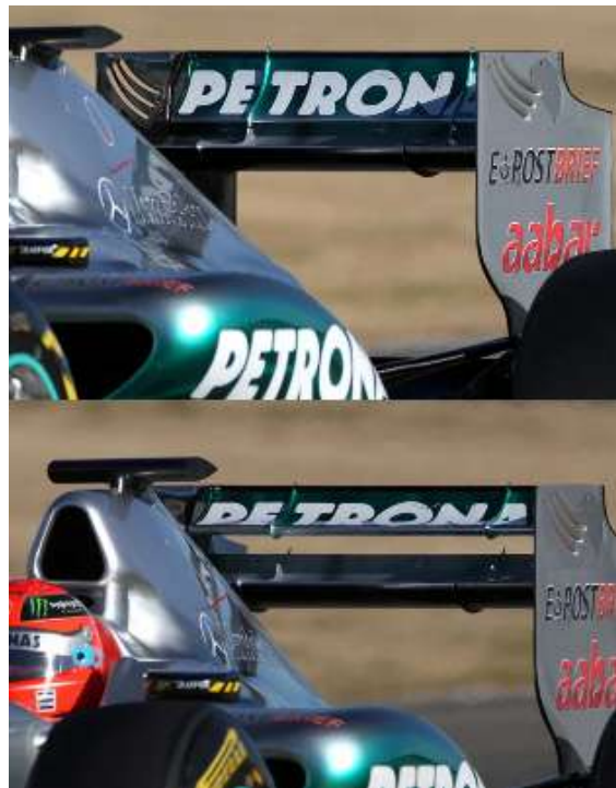
Figure 2.22: A closed rearwing is seen on top whose configuration can be exchanged to DRS configuration as seen below under certain regulated conditions
