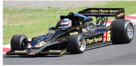
Figure 1.5: Lotus 78, the ground effect car that took advantage of side skirts to seal the floor and produce extra suction through the Venturi effect as will be explained in the chapter 2.
