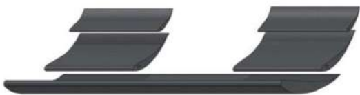
Figure 2.24: Front wing with lateral flaps individually controlled.
