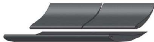
Figure 2.25: Rear wing with a split second flap to be controlled individually.
