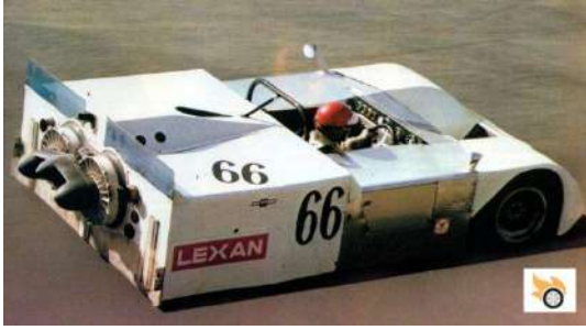
Figure 1.4: Chaparral 2J, the Sucker car , with fan mounted at the back to create suction underneath the underfloor by accelerating the airflow.
