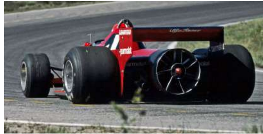
Figure 1.6: Brabham BT46, the Fan Car .
