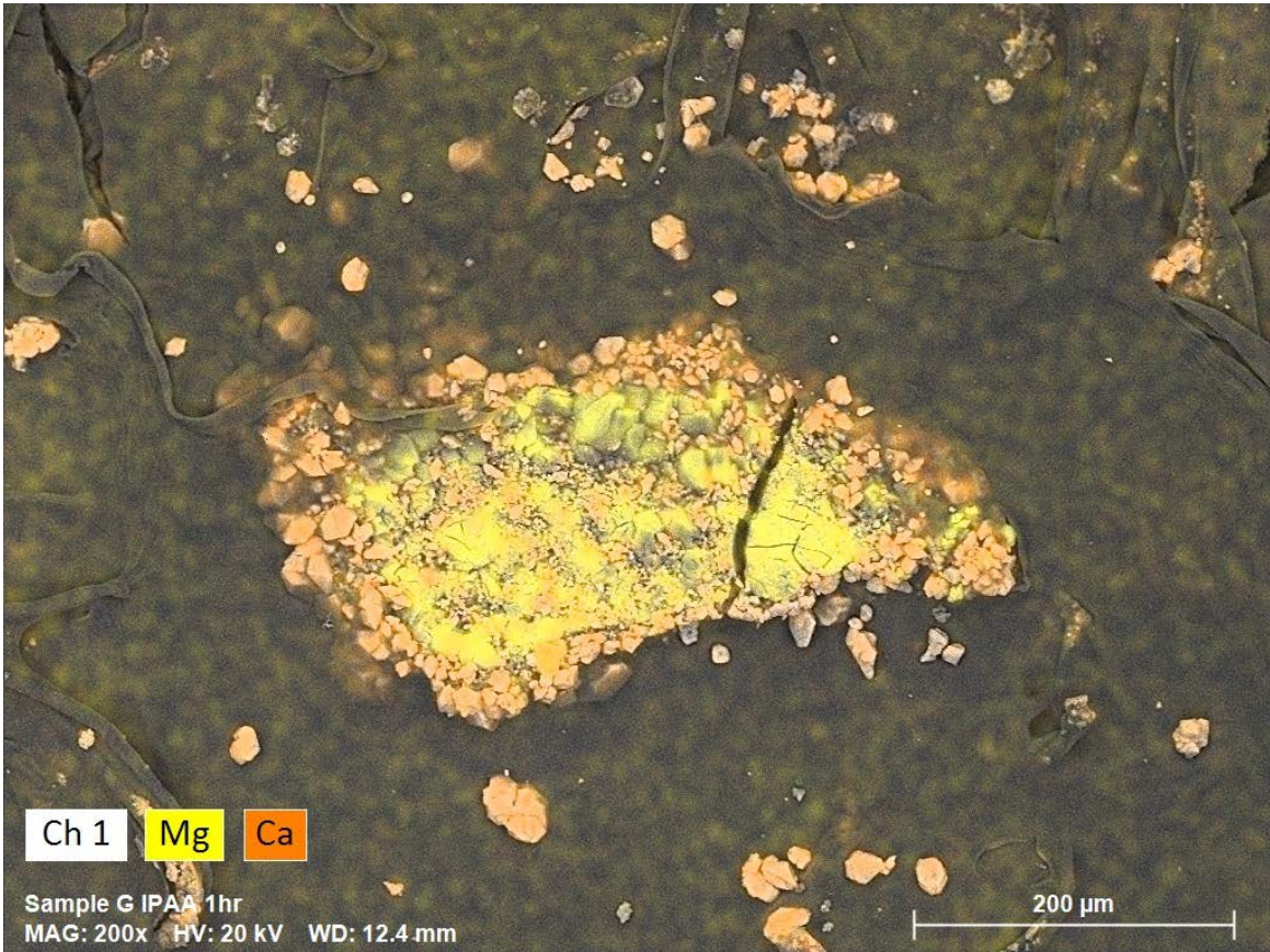
Fig. 3.30. SEM mapping image of the salts by their elements, Mg (yellow) in the center flanked on all sides by Ca (orange).
