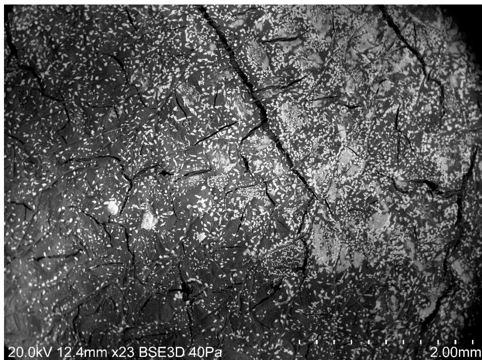
Fig. 3.56. SEM image of a large area of the untreated surface of sample 'V' almost completely saturated with salts.
