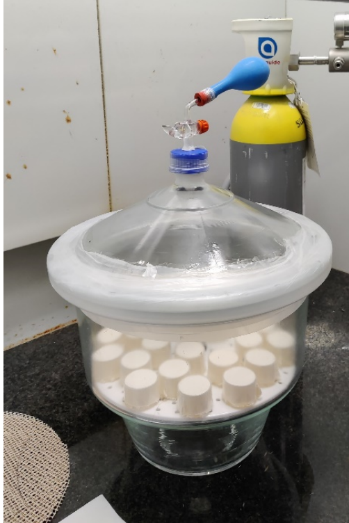
Fig. 2.3. The desiccator chamber along with the samples just after the SO 2 was introduced.
