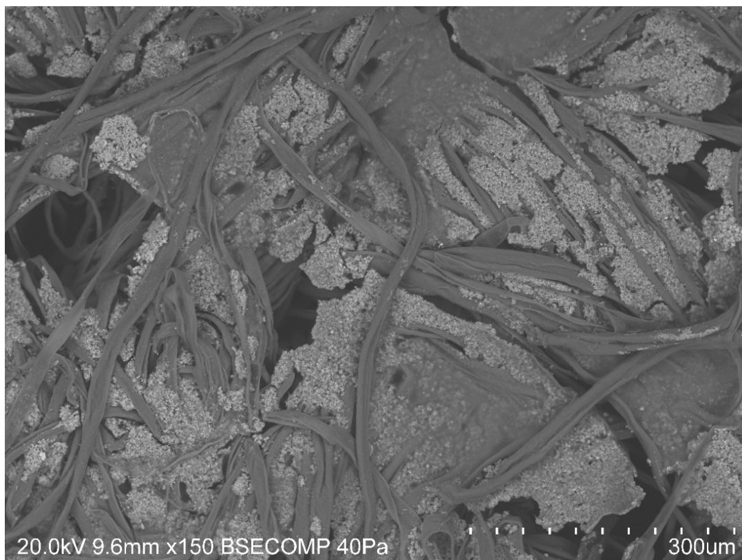
Fig. 3.39. SEM image of sample 'K', a closer look at the surface deterioration.
