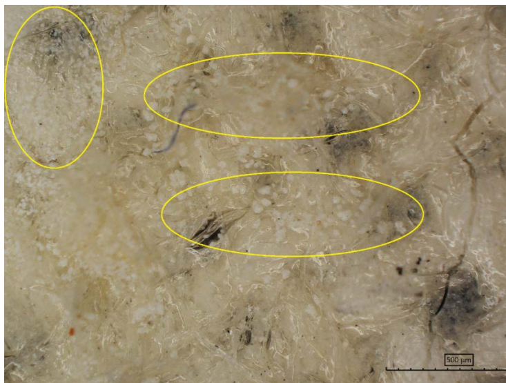
Fig. 3.25. HIROX image (140x mag.) of the untreated side of sample 'F', note the large number of salts present throughout the surface.
