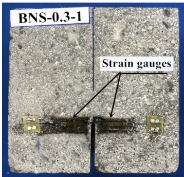
(a) Arrangement of strain gauges
