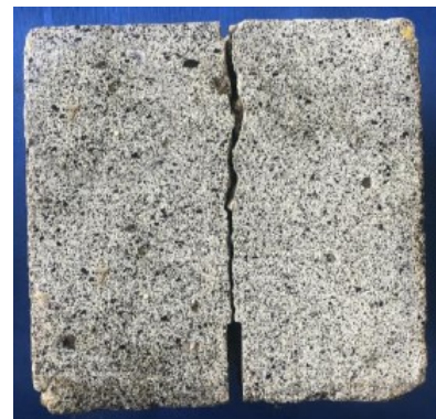
(b) Failure pattern for a_0/D = 0.2
