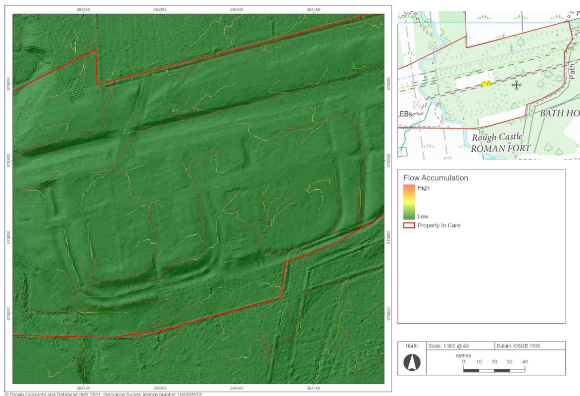
Figure 56 Flow accumulation for Rough Castle. Red indicates a high accumulation and green low accumulation.
