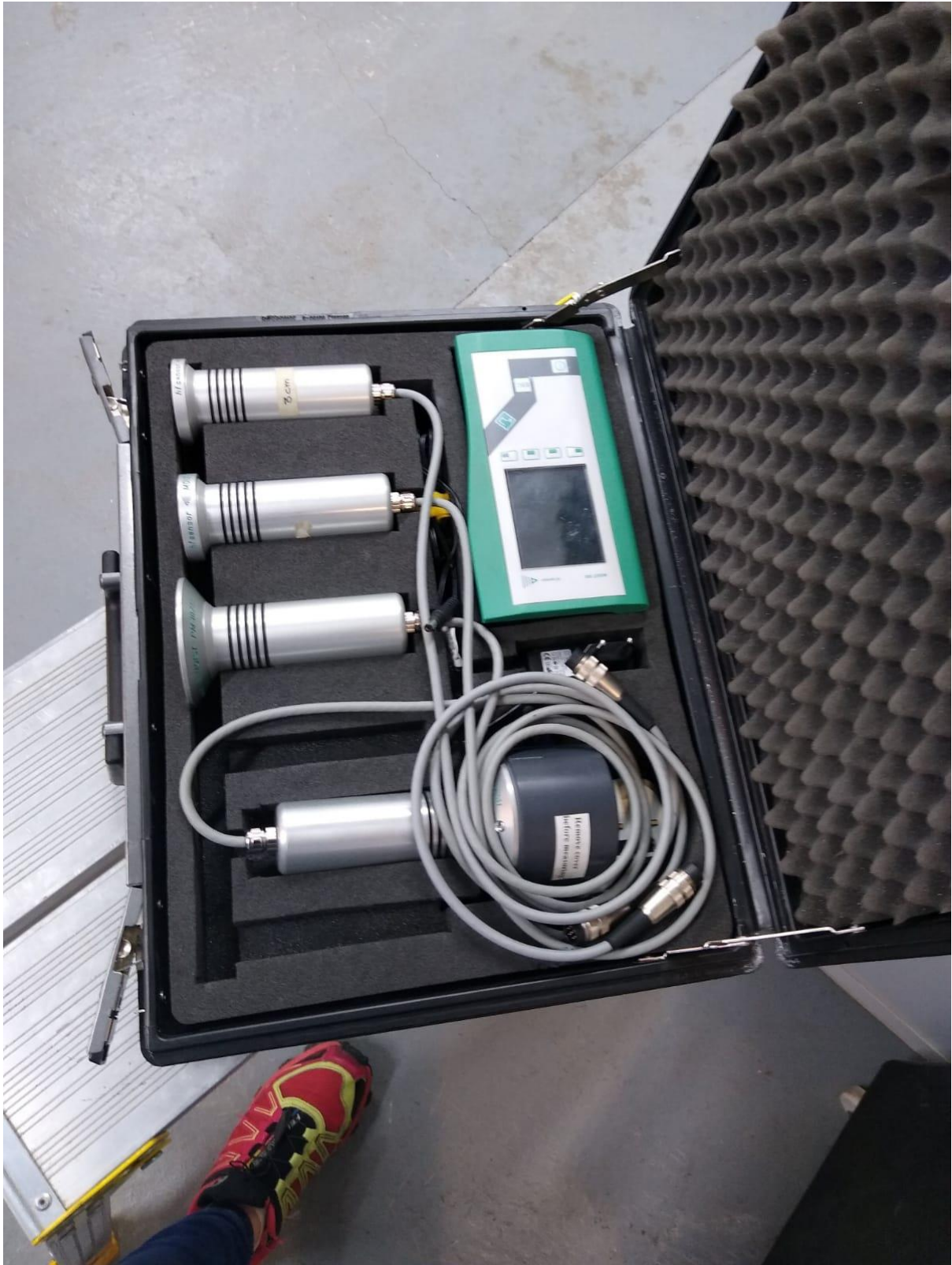
Figure 17 MMS sensors and handset within storage box. 3cm, 11cm, 30cm and 80cm sensors oriented top to bottom of figure.
