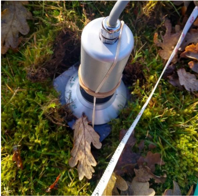
Figure 23 Sensor placed on the soil once moss had been removed, with base plate attached.
