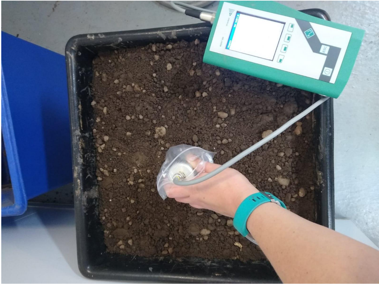
Figure 18 Test soil profile, with 3cm sensor and handset
