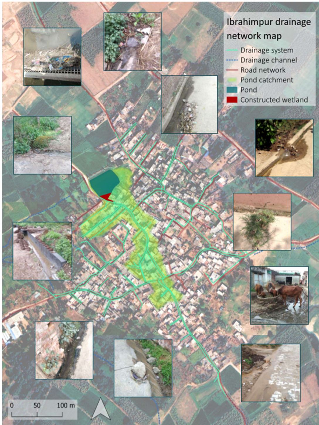
Figure 6.9 - Ibrahimpur catchment and drainage mapping. Cartography by author, based on data from site walks, embedded photographs by author, 2019-2020.
