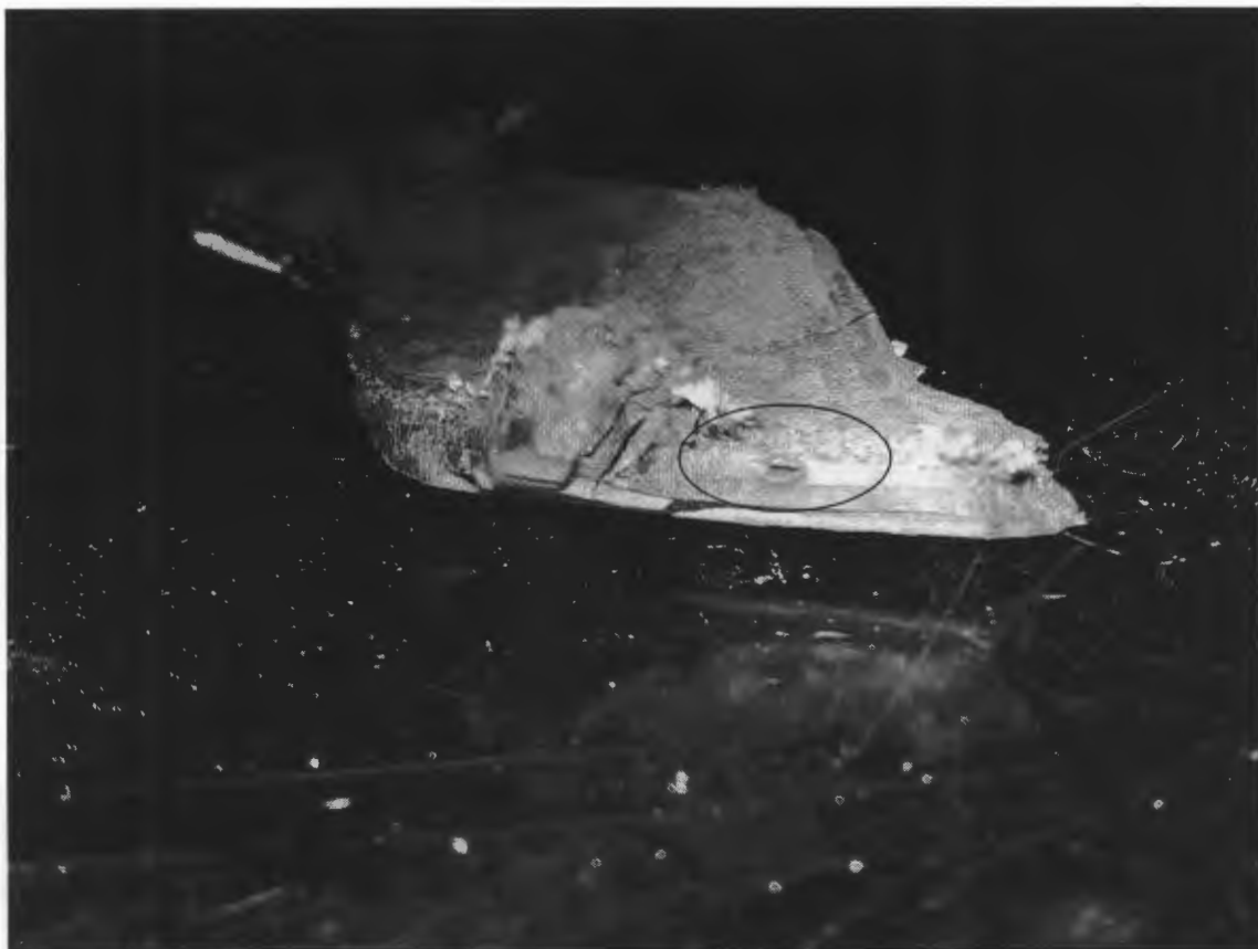
Figure 5 Photo of another heat induced pocket.
