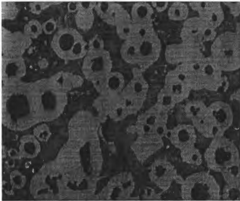
Figure 11. Structure of as cast samples 100X 4% Nital.
