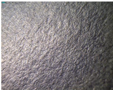
Fig. 1. The surface of aluminum sheet after rolling with office paper
