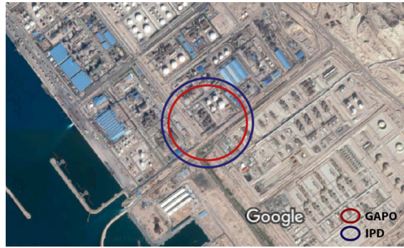
FIGURE 5: Individual risks contours (1pmpy) for GAPO compared to IPD (IPD: Initial Process Design; GAPO: Genetic Algorithm Process Optimization).
