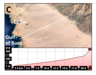
Fig. 3 (a) Google Earth map of part of the South Sinai with two locations considered for gravity-driven distributed RO shown in (b), and gravity-assisted distributed RO shown in (c). The elevation plots of the two locations are shown
