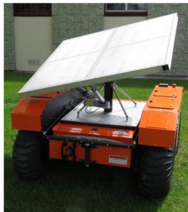
Figure 2.1.1-1: Argo J5 with the custom-built landing platform [12].
