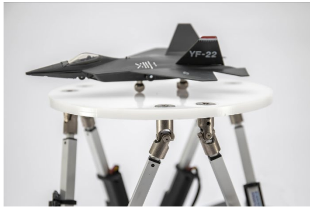
Figure 3.1-1: This figure illustrates a traditional design of the Stewart platform [23].
