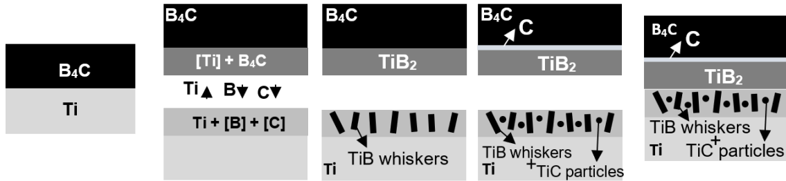
Figure 2.4. Schematic diagram of the microstructure evolution in the Ti-B 4 C system [111].
