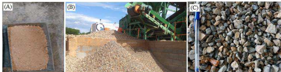
Fig. 1. Recycled aggregates: (A) fine aggregate, (B) coarse aggregate being produced and (C) large aggregate.
