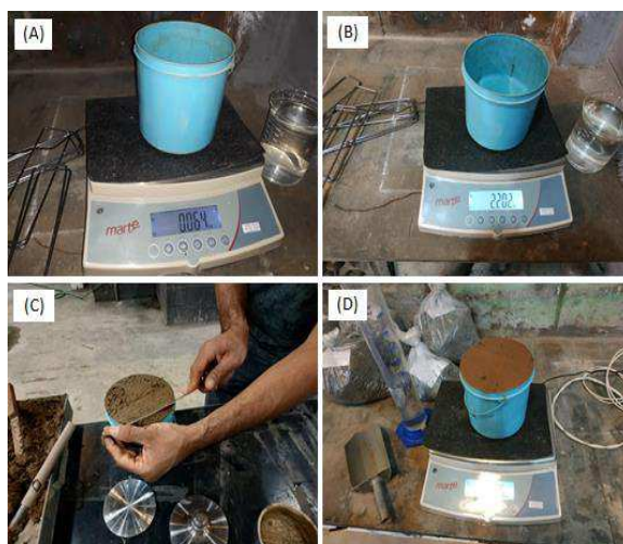
Fig. 4. Determination of density: (A) weighing of the empty container; (B) weighing of the container with water; (C) filling the container with mortar; (D) weighing of container with mortar.
