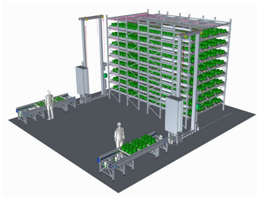
Figure 1 - Diagram of a basic Plant Factory as seen in Urban Crop Solution's website
