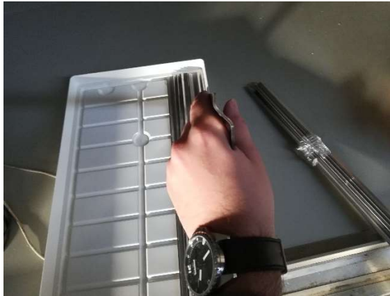
Figure 15 - Metal profiles to help guide condensate towards the plastic floor
