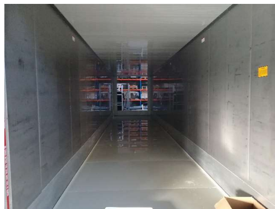
Figure 14 - Empty container with the plastic floor mounted
