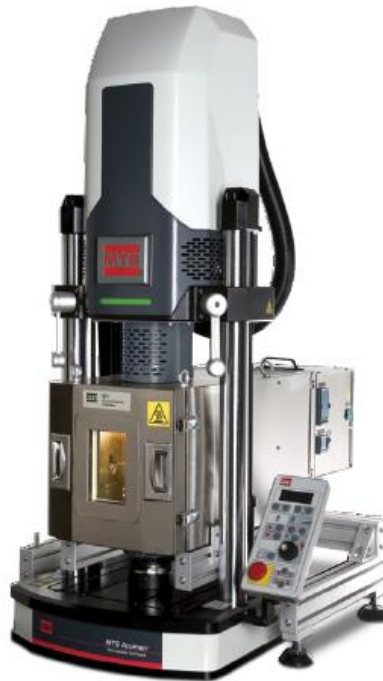
Figure 22: The final configuration of the MTS Acumen™ 3 Test System connected to the controller and the chamber.
