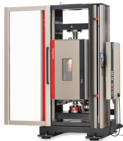
Figure 12: Representation of the Zwick/Roell Z005 machine used for hysteresis elongation tests.
