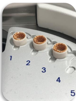
Figure 18: Samples of rayon cords in the pan, waiting to be placed on the furnace from TGA/DSC 2.
