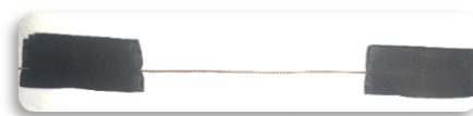
Figure 23: Example of a sample of rayon cord prepared for the dynamic mechanical analysis.
