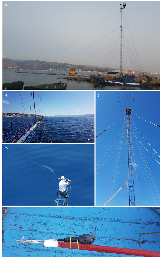
Fig. 2. Harpoon vessel and equipment used for the tagging experiment. ‘ Feluca ’ boat (a), plank (b), ‘must’ (c) harpooner during fishing operations (d) and modified harpoon consisting in a 3.5 m pole equipped with the pop-up satellite archival tag (e).
