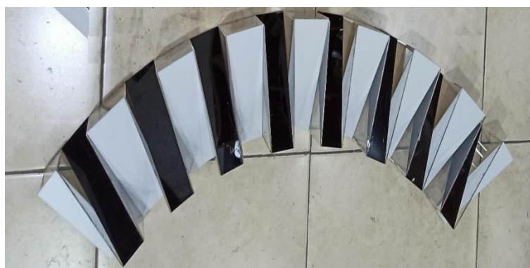
Fig. 2- Fabricated physical model of arched Pianokey weir
