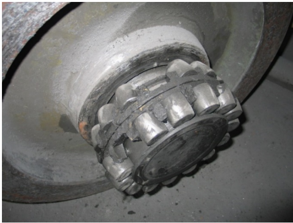
Figure 1. Coking traces of lubricant on the running wheel bearing details.
