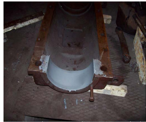
Fig. 5. Restored housings worn surfaces being in contact with rolling bearing: a) bottom housing; b) top housing.
