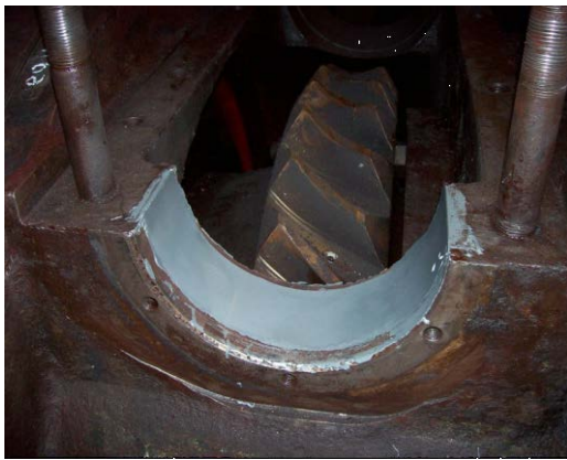
Fig. 5. Restored housings worn surfaces being in contact with rolling bearing: a) bottom housing; b) top housing.
