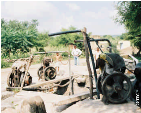
An irrigation well in Rajasthan with 3 diesel engines
