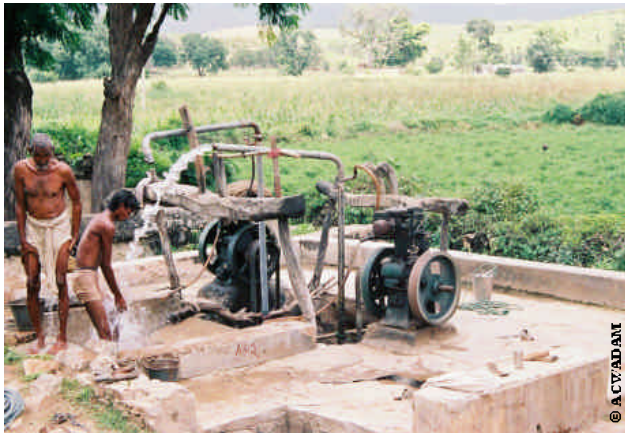
Two diesel engines pumping out water from a dug well in the Arwar basin, Rajasthan
