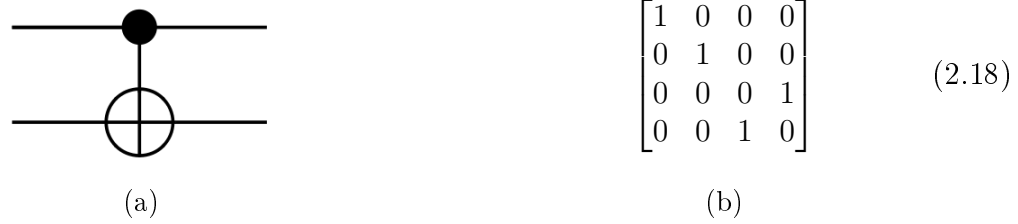
Figure 2-4: Feynman Gate: a) the CNOT gate, b) the matrix of CNOT gate
