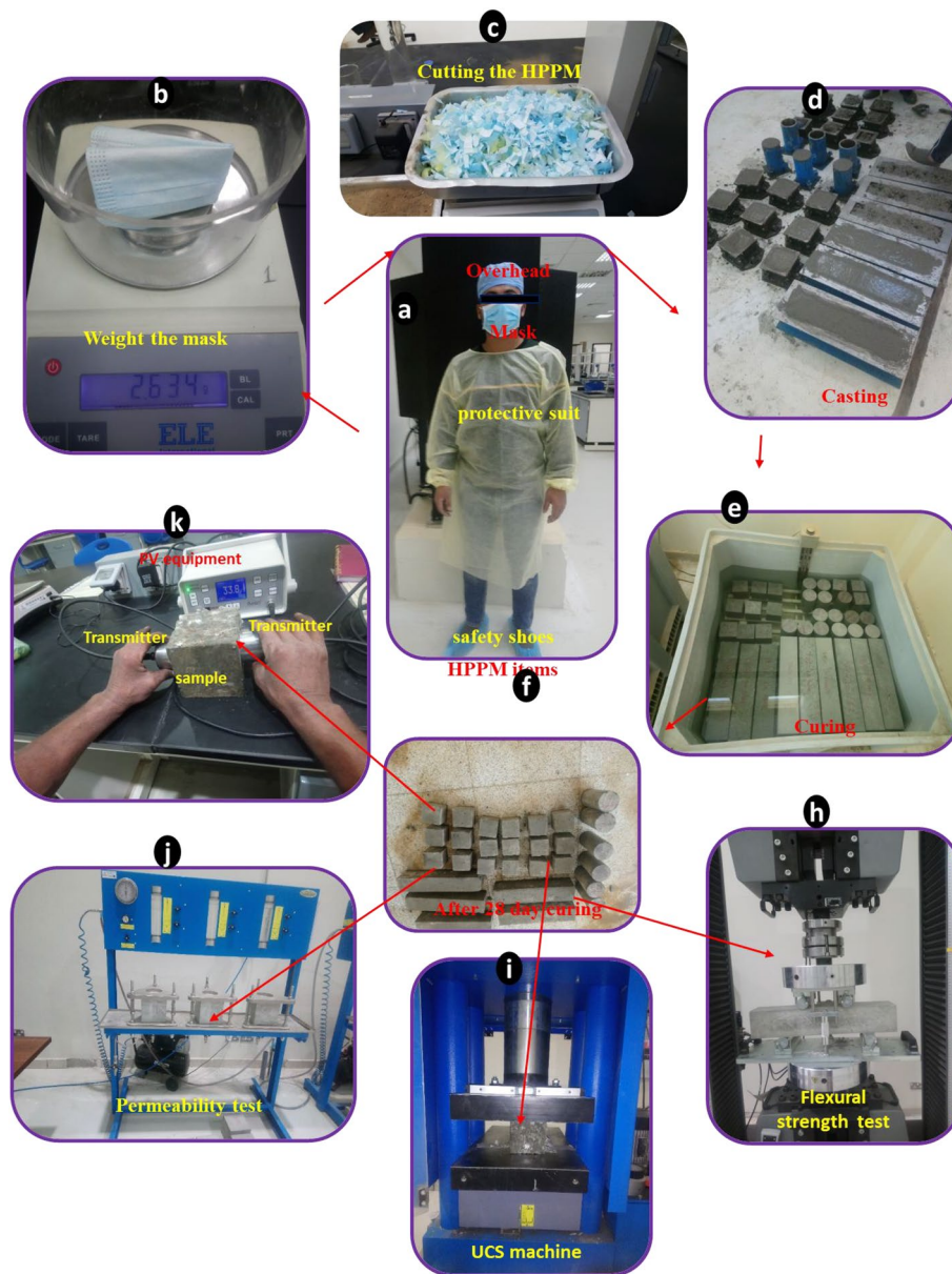
Figure 1. Experiment protocols, casting, and curing of the concrete with HPPM.
