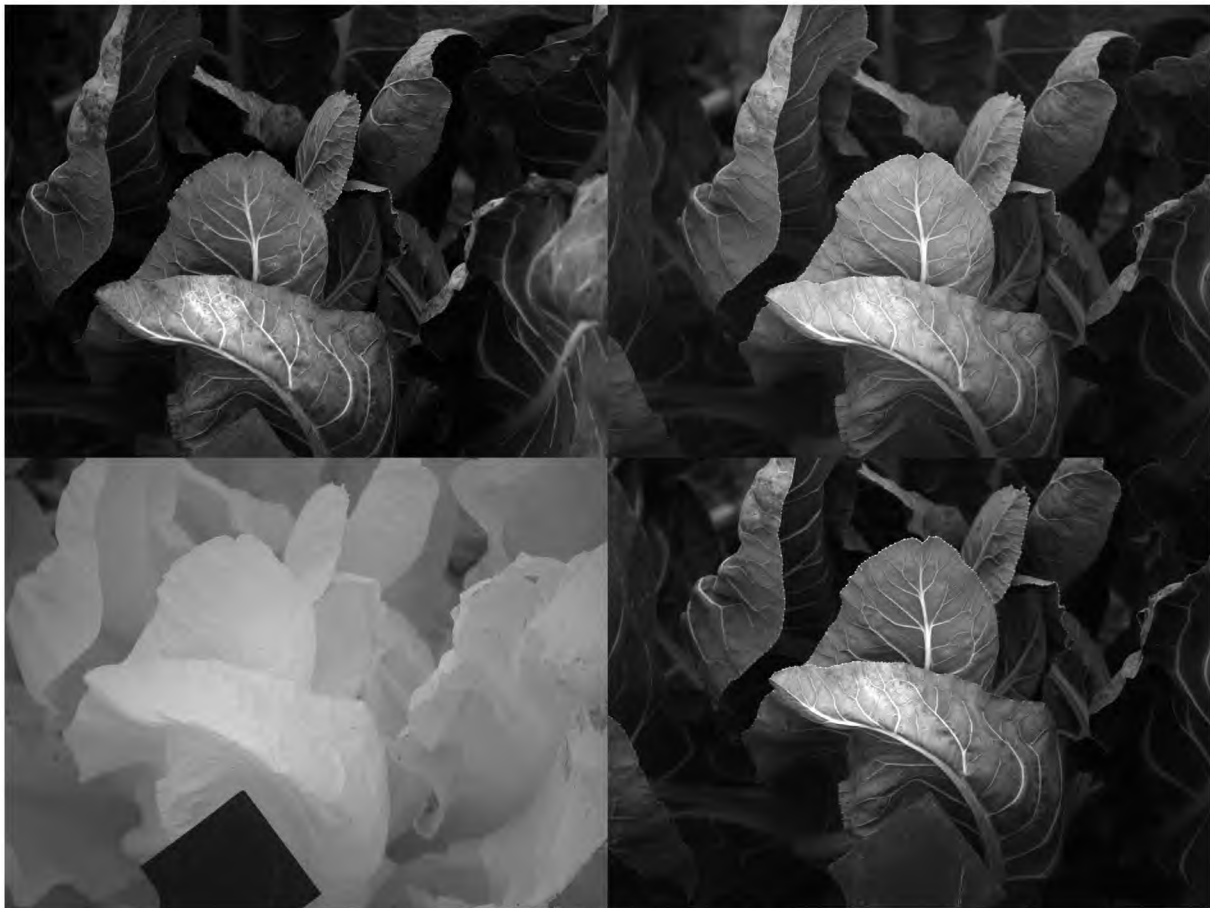
Figure 3. Agros scanner sample measurement from 4 spectral cameras—each spectral resolution 1400 \times 1200 pixels, spectral lengths: 470, 550, 850 and 640.
