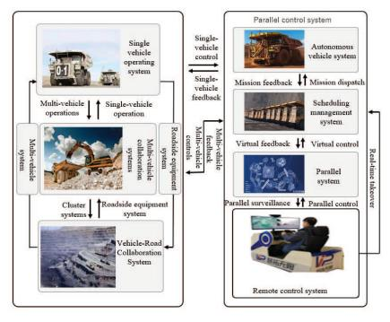
Figure 2. Schematic diagram of the parallel intelligent mining operating system.
