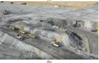
Figure 3. Implementation of parallel mining: (a) parallel control center; and (b) collaborated autonomous mining trucks.
